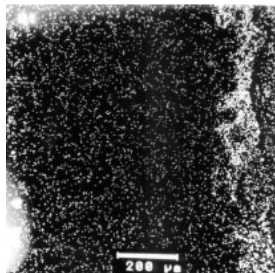
Fig. 6 Cross section of a field-tested reheat tube with the coating system Ni20Cr/Ni20Cr-50FeCr showing x-ray mapping of Ni, Fe, Cr, V, and Al. (M, metal; R1, Ni-20Cr; R2, Ni20Cr-50FeCr).
